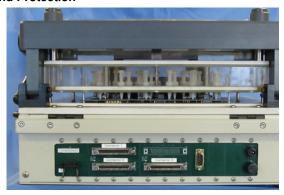
Microlynx' unique Modular Back Plane provides an easily accessible area for all interconnections between the test fixture and the rest of your test equipment. You do not need to access the inside of the fixture to change cables.
